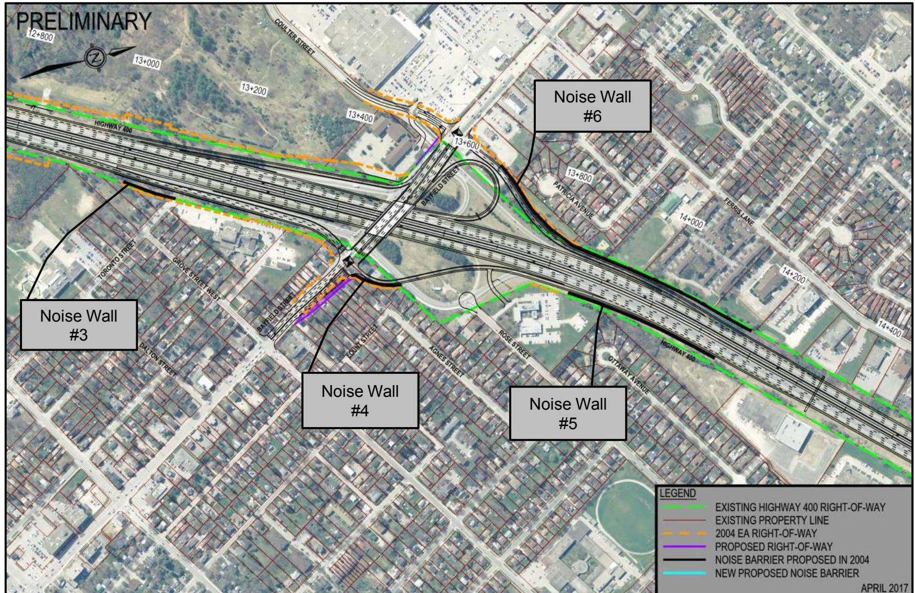
Figure 31: Recommended Noise Barriers - Locations 3, 4, 5 and 6
